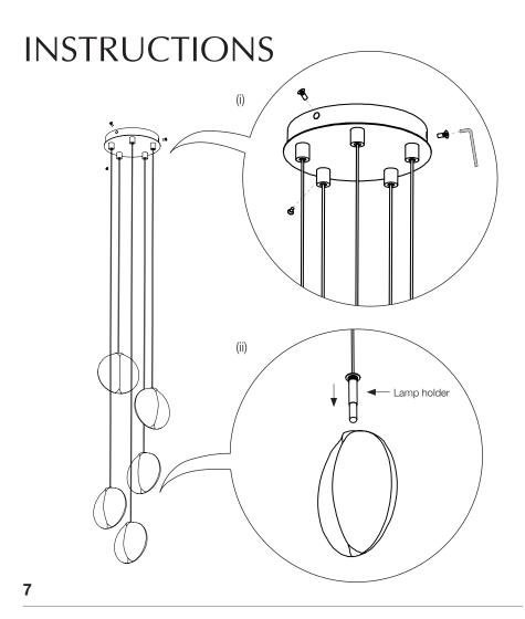
(i) Tuck the wiring neatly into the canopy. Affix the front plate to the back plate using the Allen wrench and the screws previously saved. Ensure cover is properly screwed down.
