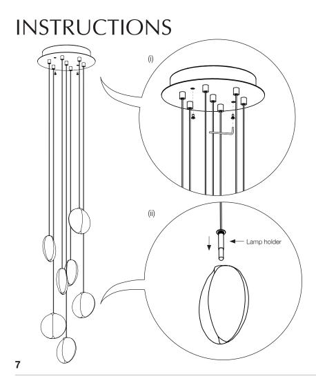
(i) Tuck the wiring neatly into the canopy. Affix the front plate to the back plate using the Allen wrench and the screws previously saved. Ensure cover is properly screwed down.
